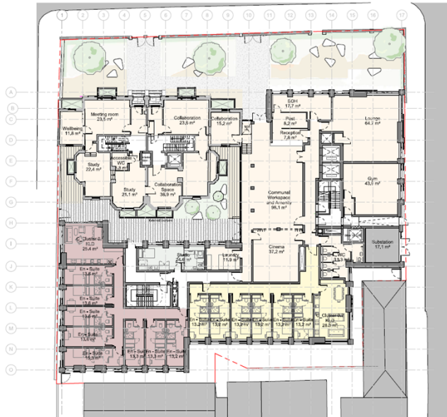
Proposed layout plan indicating link to existing Grade II listed building to Moss Lane East frontage
